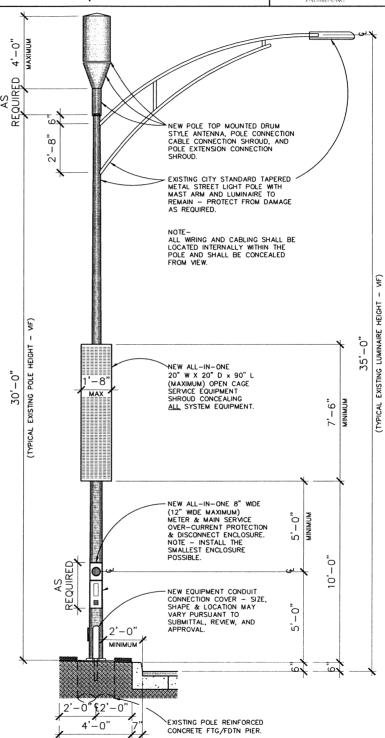
Appendix-B: Standard Configuration - Existing Street Light Pole with Pole Mounted System
