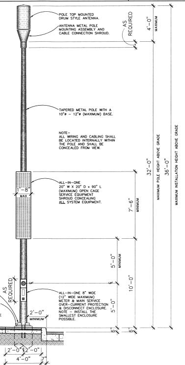
Appendix-C: Standard Configuration - New Tapered Metal Pole with Pole Mounted System
