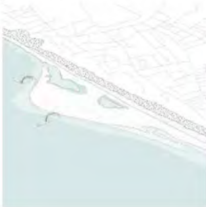
Fig. A.5 Dredged sand is placed along-shore in a mega-nourishment.
