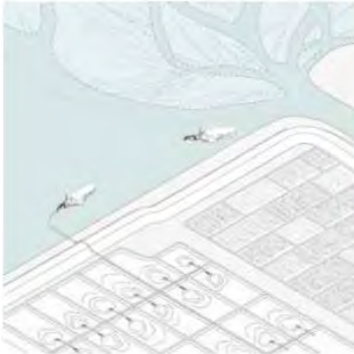
Fig. D.5 Dredgers remove sediment from areas of problematic buildup.
