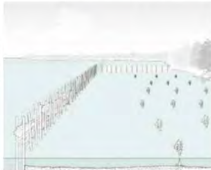
Fig. B.6 Permeable structures attenuate waves; sediment settles behind.
