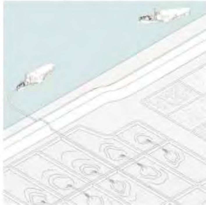
Fig. D.6 Fine, silty sediment is pumped into the ripener.
