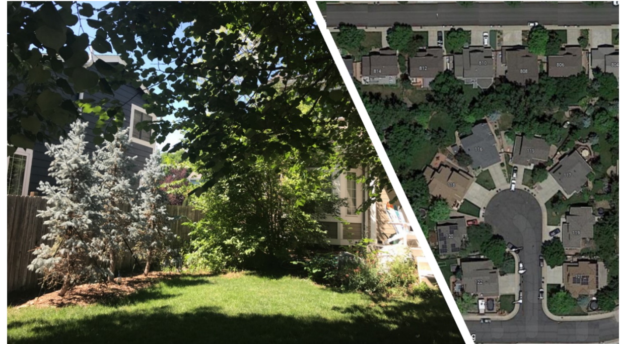
Example of single-family-residences with 5–8 feet to property lines and significant overgrown vegetation. Both homes are vulnerable to spot fires from embers or structure-to-structure fire spread
